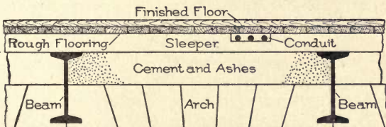
Fig. 32. Running Conductors Concealed Under Floor in Fireproof Building
